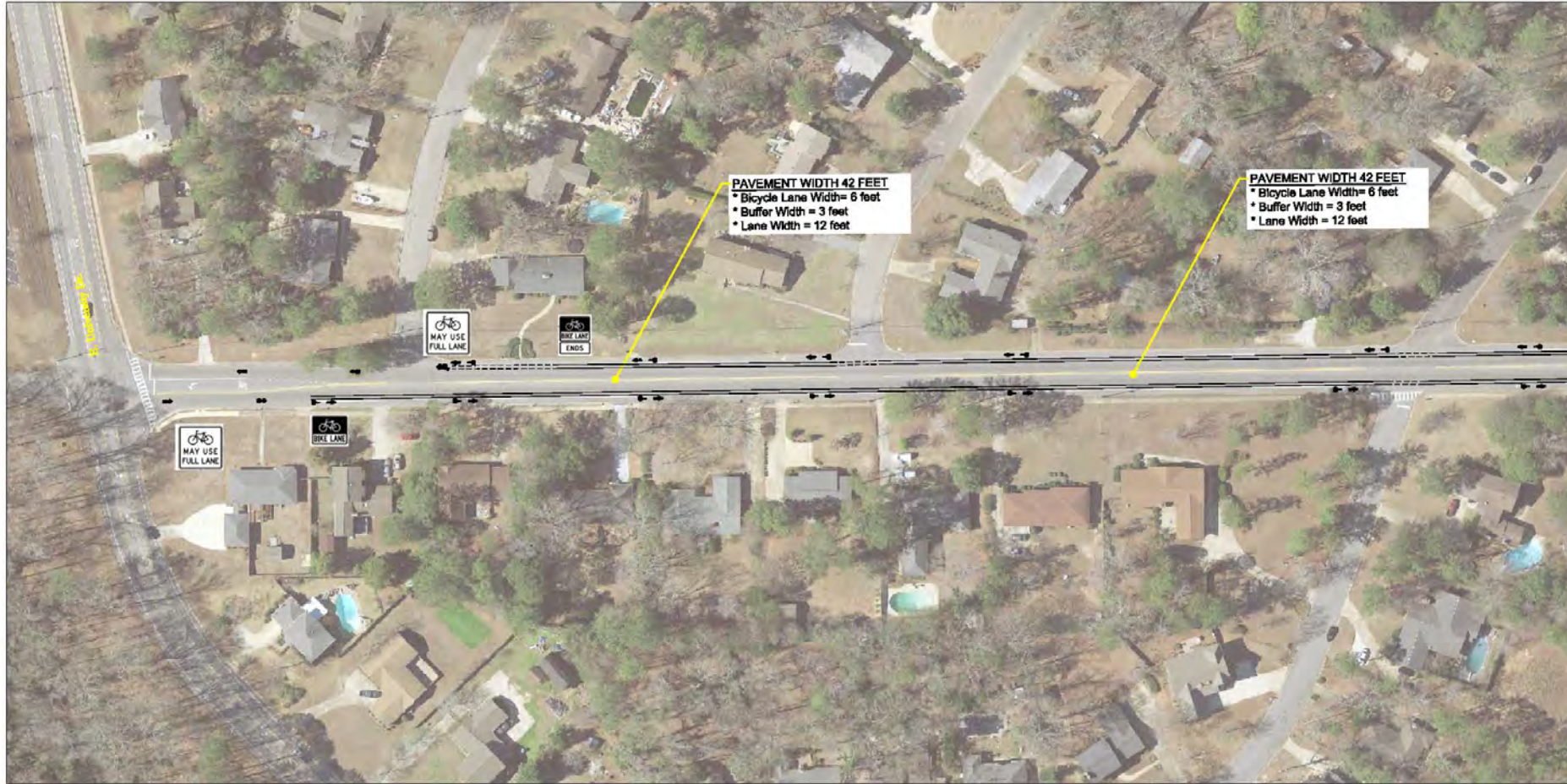
Dean Road (3-Lane Cross-section with Bicycle Lanes) at East University Drive South
