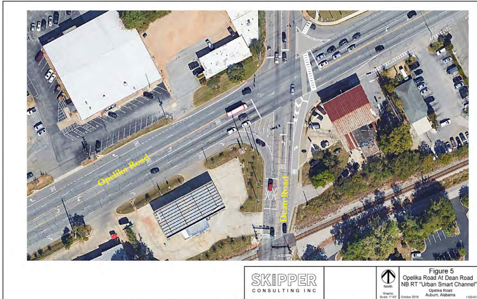
Figure 5 – Opelika Road at Dean Rd. – Modify NB Right Turn Lane with "Urban Smart Channel" Design
