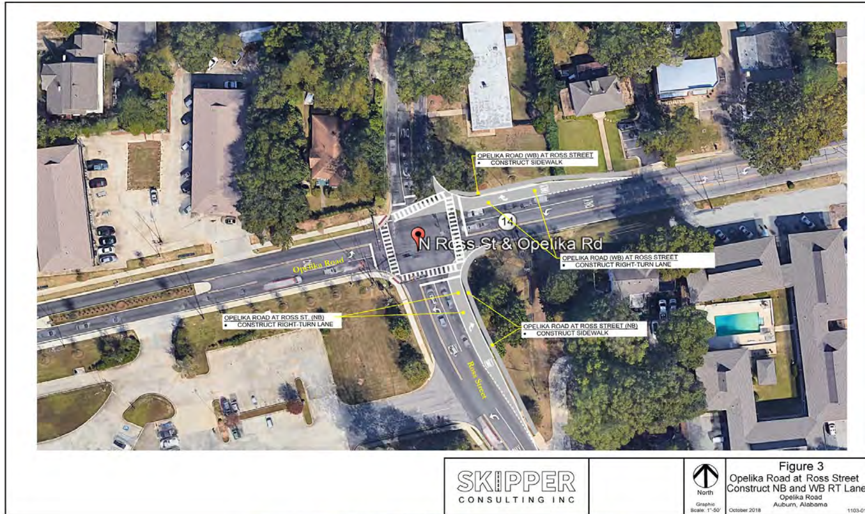
Figure 3 – Opelika Road at Ross Street NB and WB Right Turn Lane Improvements
